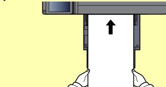
• After printing starts, catch the paper when it is output so that it does not fall.
